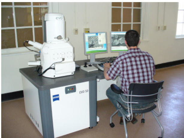
The new Carl Zeiss EVO-50VPX Scanning Electron Microscope (SEM) located in Butterfield 205.
