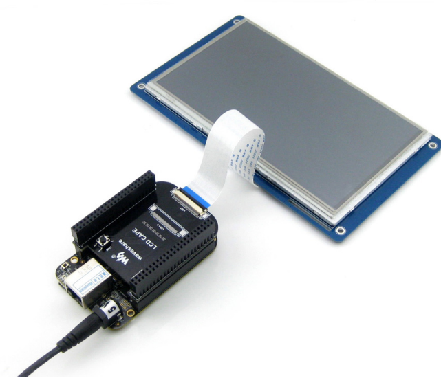
Figure 2: An LCD display for the BeagleBone Black [19].
