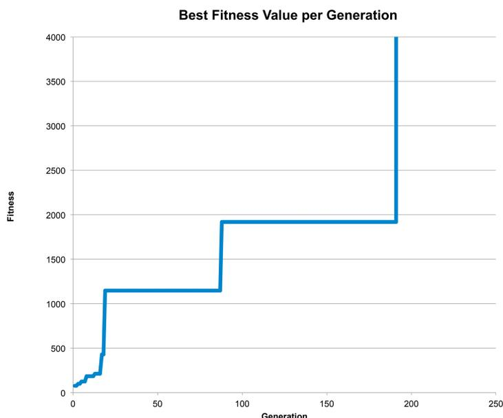
**Figure 5 (left).** This graph shows the best fitness values per generation over the course of an experiment. At generation 192, the fitness jumps from 1,920 to over 40 trillion. This astronomical number indicates a serious bug in the simulation code. This results in individuals with false fitness values and spoils the evolutionary process.
