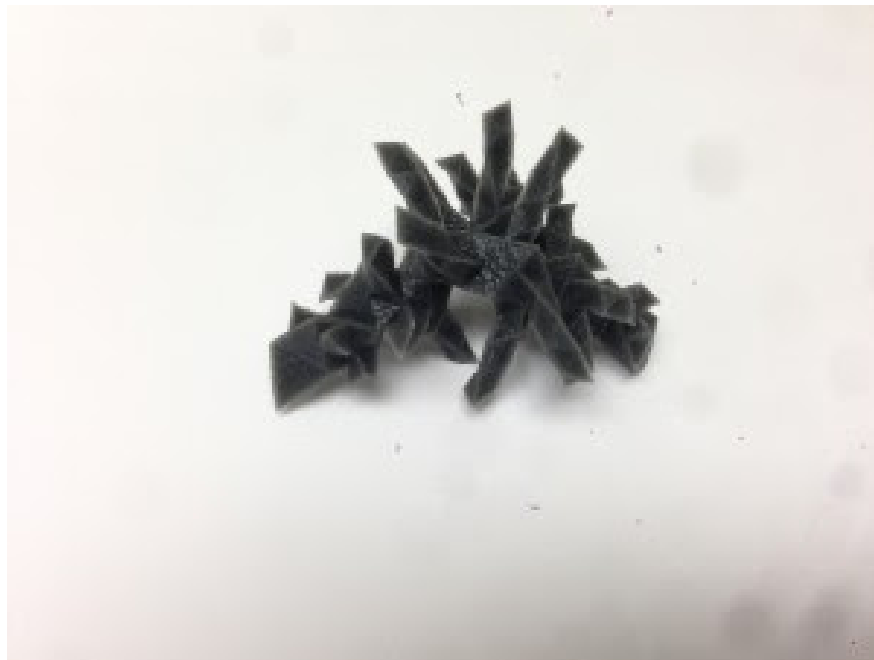
Figure 2: A 3D printed robot designed using the above algorithm. Electrical components such as wires and vibrational motors will be inserted into the robot mid-print.
